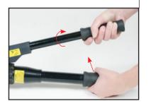
Automatic release with audible "click" in the event of verload. Piston return by rotation of the moveable handle.
