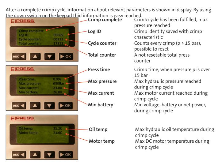
If any of the parameters above, press time, pressure, current, voltage, oil temp or motor temp is out of preset limits there will be an error message with information about the actual problem. When a crimp cycle has been started but not completed within 60 sec, a message "Time out" will be shown in the display. All faulty messages can be cleared in "Active faults" menu.
