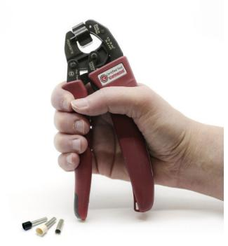
PEB0110T18 is a new tool for crimping end sleeves that are up to 18 mm long in a single crimp. The crimp tool is self-adjusting, thus ensuring quality. Front feed makes the tool user-friendly and convenient in confined applications. The crimping tool is tested for 50,000 crimps without calibration and is thereby "life-time-calibrated".
