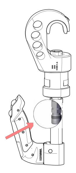
Risk for oil leakage in the quick coupling, see the area the arrow shows. It's is very important that the Ergo pipe is not loosen and it has it's original position to prevent sudden oil leakage.
