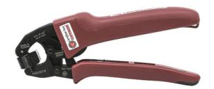
PEB0110T18 is a new tool for crimping end sleeves that are up to 18 mm long in a single crimp. The crimp tool is self-adjusting, thus ensuring quality. Front feed makes the tool user-friendly and convenient in confined applications. The crimping tool is tested for 50,000 crimps without calibration and is thereby "life-time-calibrated".
